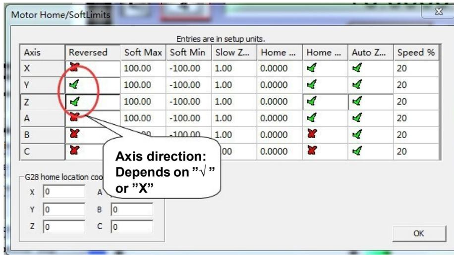
The HOME location can be set to any corner of the CNC as determined by the checkmarks for each axis. The **X** chooses the default direction and the **Checkmark** chooses the opposite.
