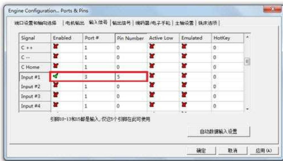
On the Diagnostic Screen, the indicator marked Input #1 will illuminate whenever the switch on Port3-IN5 is closed.
