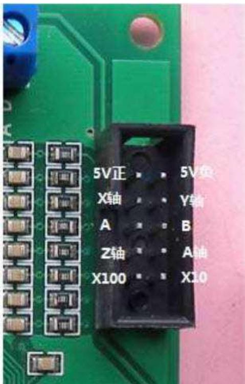
The auxiliary inputs are all rated for a maximum of 5Volts. 3.3 Volts is preferred. The interface is as follows.
